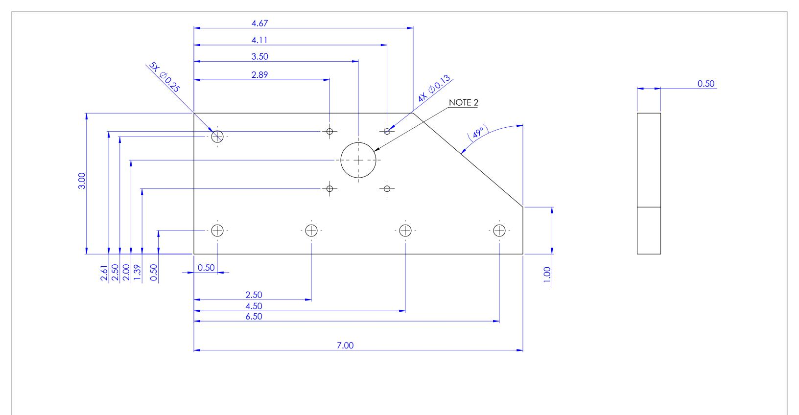
NOTE 1: DRAWING MAY BE USED AS TEMPLATE AS LONG AS IT IS NOT SCALED DURING PRINTING NOTE 2: HOLE PATTERN AND CUT OUT FOR NEMA 17 STEPPER MOTOR
