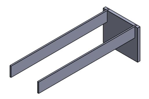
NOTE 1: STRINGERS ARE EPOXIED OR SOLDERED IN PLACE. NOTE 2: THIS IS THE FRAME, TO PROVIDE GOOD CONTACT ON THE RECEIVER AN EPOXY WEDGE IS MADE TO FILL THE GAP
