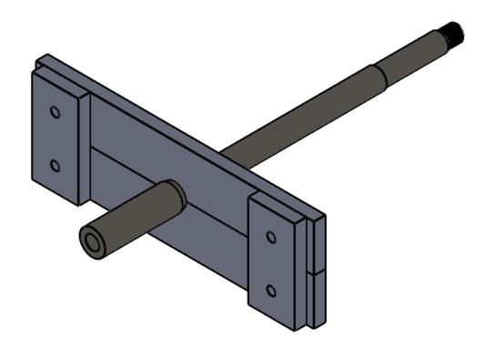
NOTE 1: CONSTRUCTION IS ENTIRELY 3/8X1.5 MILD STEEL STOCK NOTE 2: FOUR 1/4-20X 2IN BOLTS ARE NOT SHOWN BUT ARE REQUIRED TO COMPLETE ASSEMBLY
