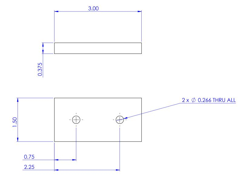
NOTE: HOLE SIZE SHOULD PROVIDE SUFFICIENT CLEARANCE FOR A 1/4X20 BOLT
